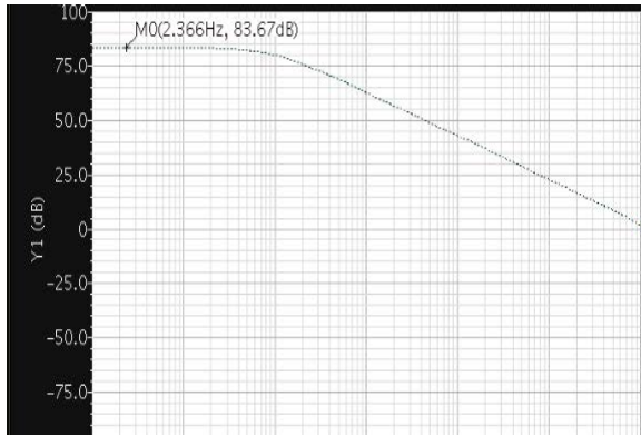
Fig9 .Dc Gain of Op-amp
